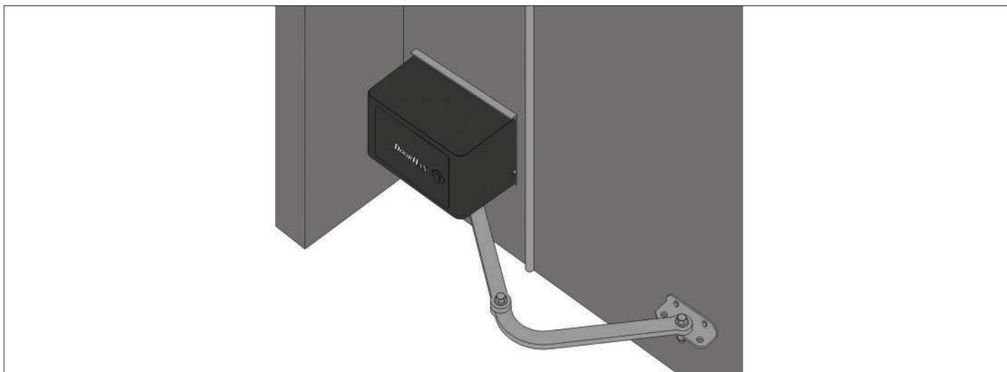
МОНТАЖ НА КОЛОНУ ОТКРЫТИЕ НАРУЖУ / INSTALLATION ON COLUMN, OPENING OUTSIDE
