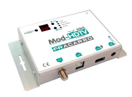
The MOD-HDTV MINI is a high quality DVB-T "Home" indoor digital modulator which accepts one HDMI signal source and converts it into one RF DVB-T channel on its output. The excellent specs (Full HD 1920\*1080-30p) and modulation quality (MER~35dB) renders the MOD-HDTV MINI the economic and ideal solution for distributing HD signals coming from e.g. a laptop or CCTV system in a domestic coax network using the DVB-T technology.
